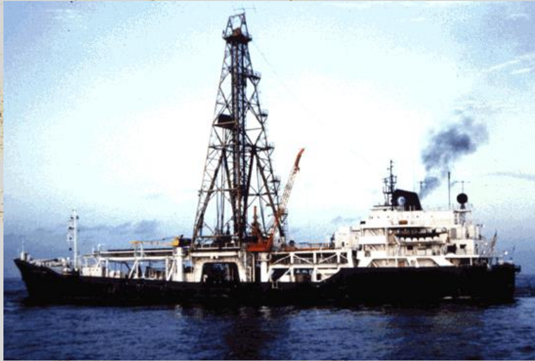
Above: The Glomar Challenger was the first research vessel specifically designed in the late 1960s for the purpose of drilling into and taking core samples from the deep ocean floor. Right: The JOIDES Resolution is the deep-sea drilling ship of the 1990s (JOIDES= Joint Oceanographic Institutions for Deep Earth Sampling). This ship, which carries more than 9,000 m of drill pipe, is capable of more precise positioning and deeper drilling than the Glomar Challenger. (Photographs courtesy of Ocean Drilling Program, Texas A & M University.)
