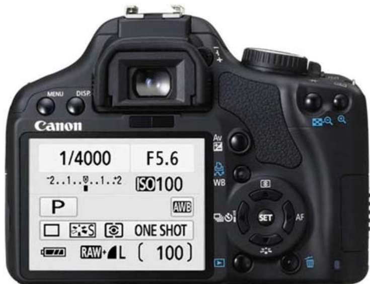
Digital camera set to 1/4000 of a second at f/5.6, with 100 exposures remaining.
